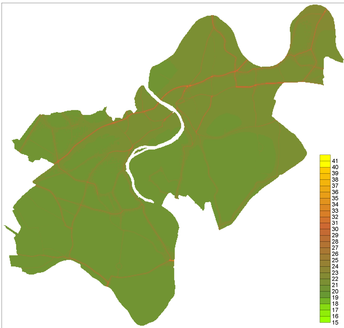
Figure 2: Modelled PM 10 concentrations in LBRuT for 2015. (Modelled by ERG from 2010 data) Annual Limit = 40ug/m 3
