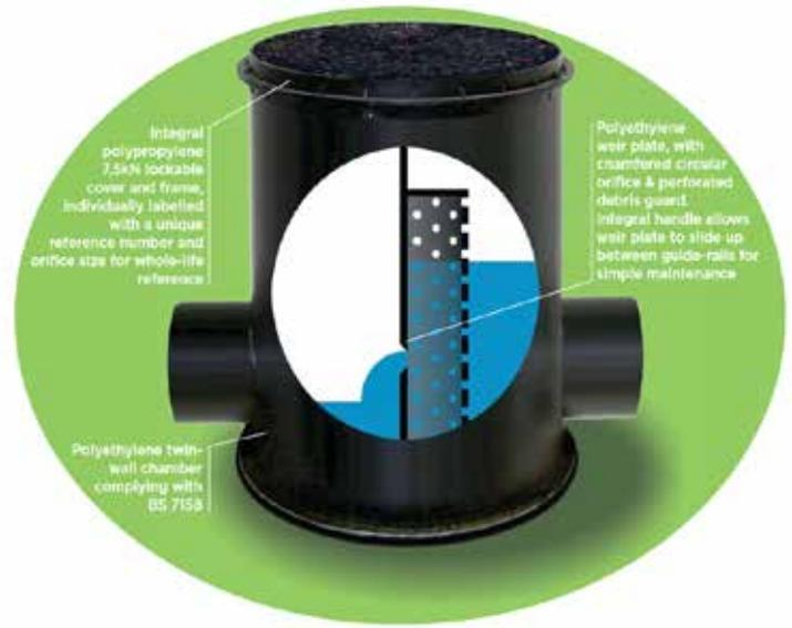
Figure 7 Example protected orifice flow controls with removable screen box (for cleaning) and with removable weir plate and perforated debris guard (for cleaning)
