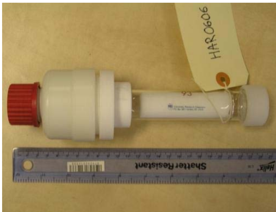
Figure D: Photograph of Particulate/Vapour-Phase Filter and PUF Sampler used in the project.
