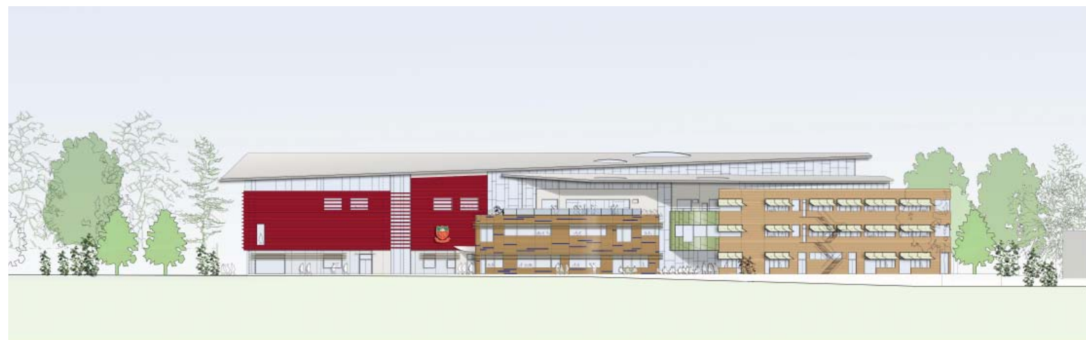
Illustrative elevation of the proposed school from the Broom Road Recreation Ground and partly from Trowlock Island illustrating potential materials, heights, roof and fenestration. This elevation seeks to illustrate the different materials and textures that would appear from the outside of the school.
