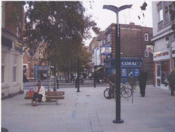
Scroll bench, Sheffield cycle stand and LG lighting set in York stone
