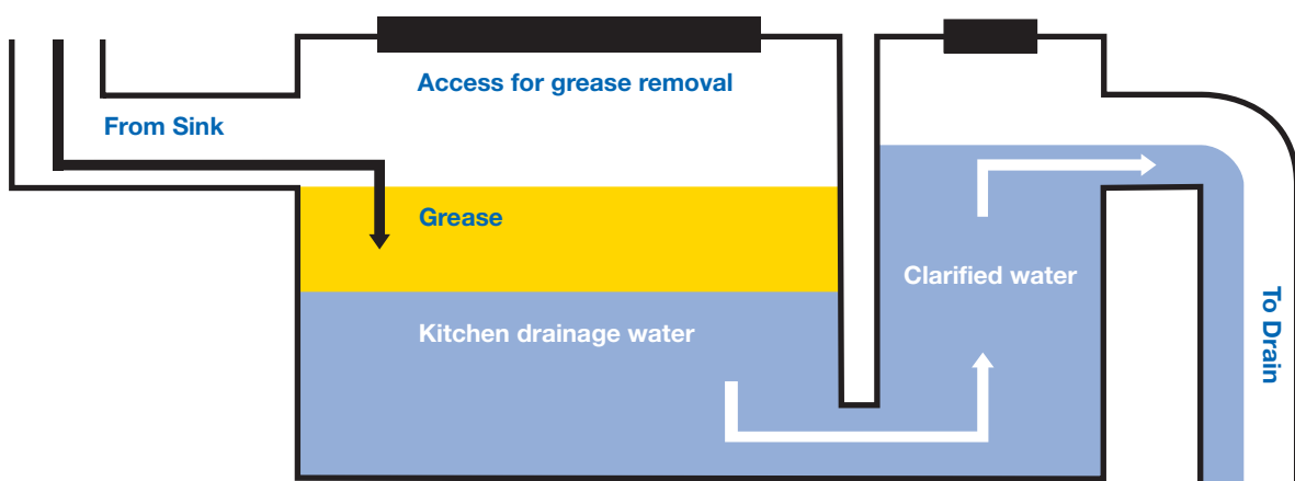
Diagram of an "under-the-sink" grease trap
