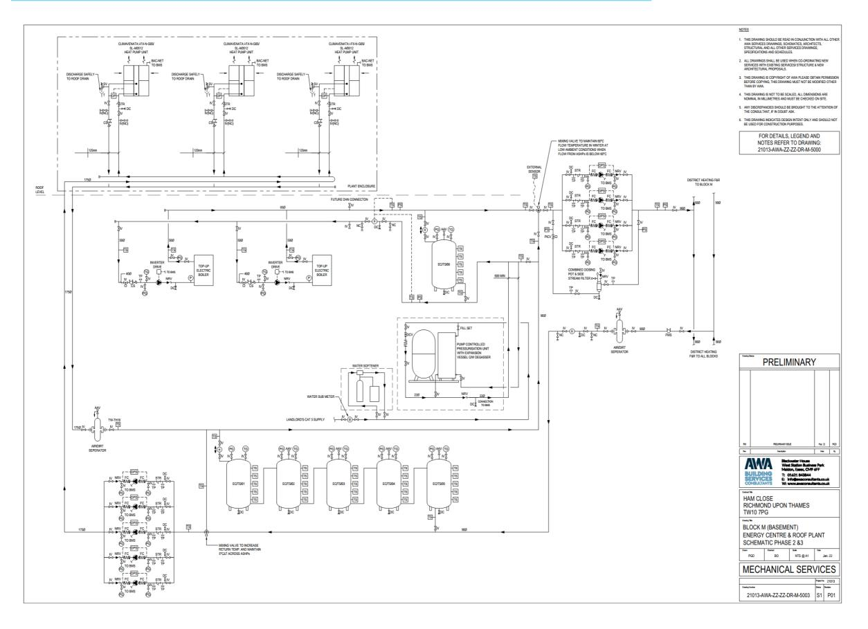
Figure 28 - Energy centre schematic, showing future DHN connection point (AWA drawing 21013-AWA-ZZ-ZZ-DR-M-5003)
