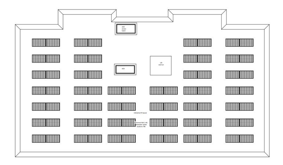
Figure 10 - Block D Roof Layout
